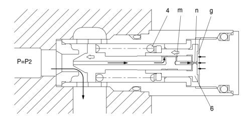
When piston(6) hits the bottom of bushing(7), it stops moving to the left any further. As the result, the pressure in chamber(g) equals(Ps).
