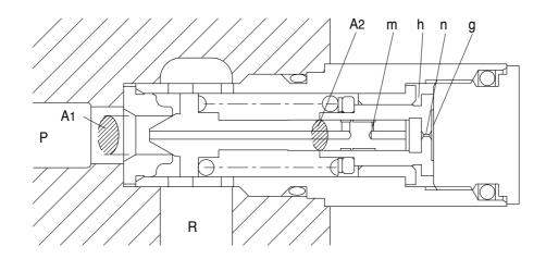
When hydraulic oil pressure( $P \times A_1$ ) reaches the preset force(FsP) of spring(4), the plunger(3) moves to the right as shown.
