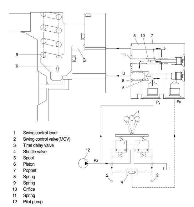
c. When the swing control(1) lever is set the neutral position, the spool(5) returns right in the time delay valve(3).
