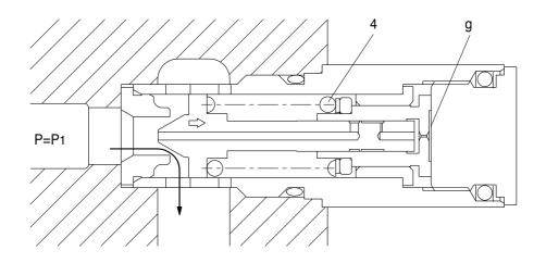
The oil flow chamber g via orifice m and n. When the pressure of chamber g reaches the preset force(FSP) of spring(4), the piston(6) moves left and stop the piston(6) hits the bottom of bushing(7).
