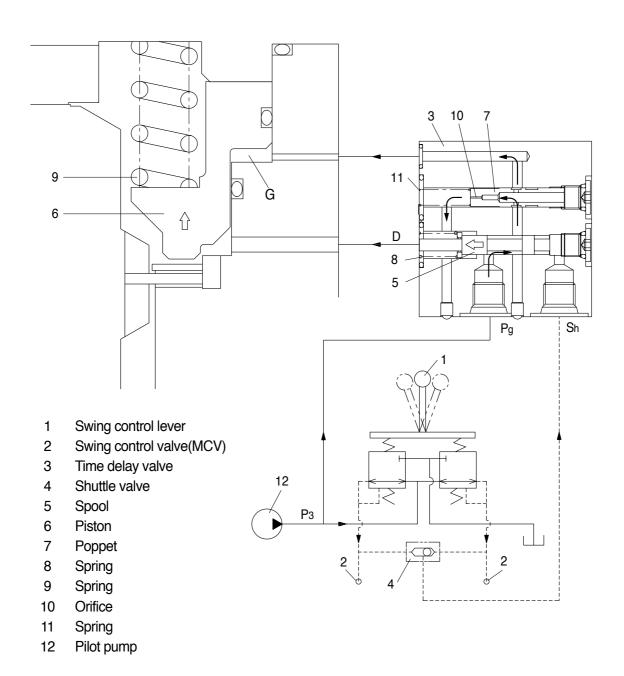
b. Meantime, the oil pressure of port D balance with the preset force of spring(11), the pressure of chamber G keeps constant pressure.
